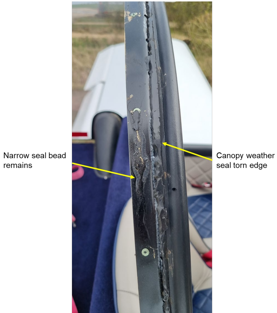
Figure 2 Dis-bonded area and canopy seal on the hoop frame
