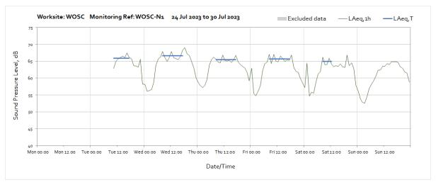
Note: Missing data from the beginning of July until 12:00 Tuesday 25<sup>th</sup> July was due vegetation overgrowth blocking the monitoring station solar panels leading to depletion of the monitor battery. The area has since been cleared of vegetation with view of minimising loss of data in the future.
