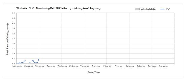
Note: Missing data to the end of the month was due to depleted monitor battery, the monitor is planned to be swapped with a new one.
