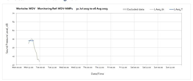
Note: Missing data until 12:00 on Monday 31<sup>st</sup> July was due to damage to monitor power cable which has now been replaced.
