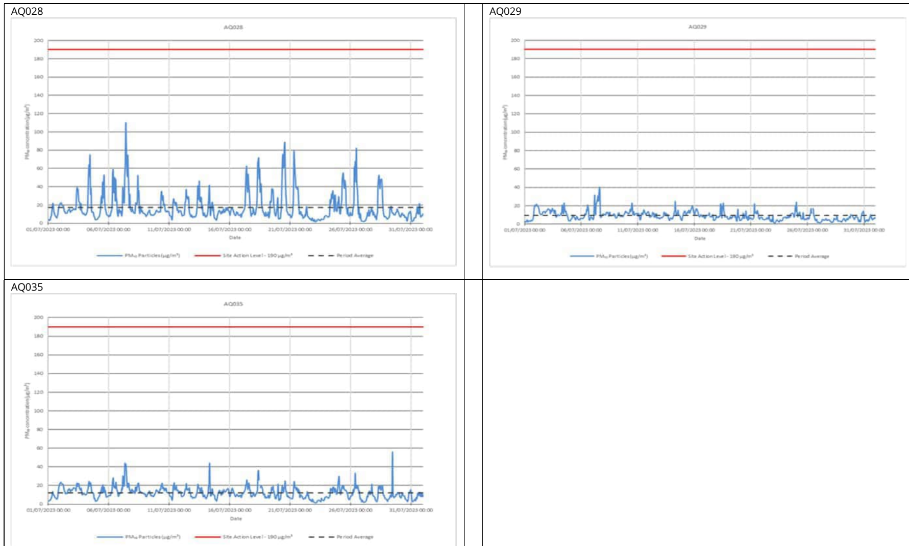
Figure 3: Construction dust 1-hour mean indicative PM 10 concentration for dust monitors
