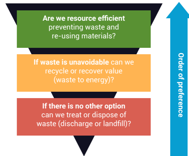
FIGURE 6: TAQA UK'S WASTE DISPOSAL HIERARCHY
