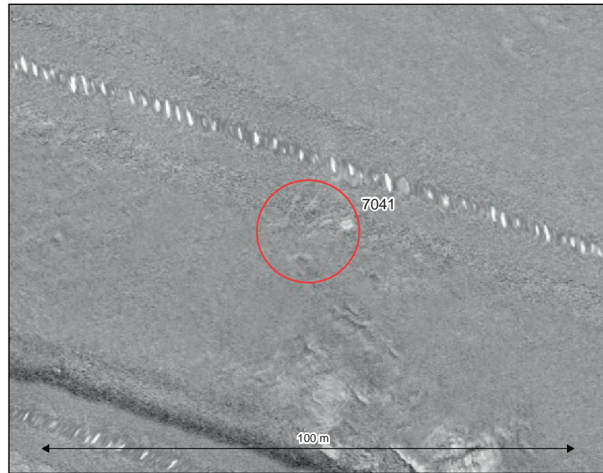
Pseudo SSS mosaic image of debris field 7041 , measuring 14.5 x 10.4 m, looking north
