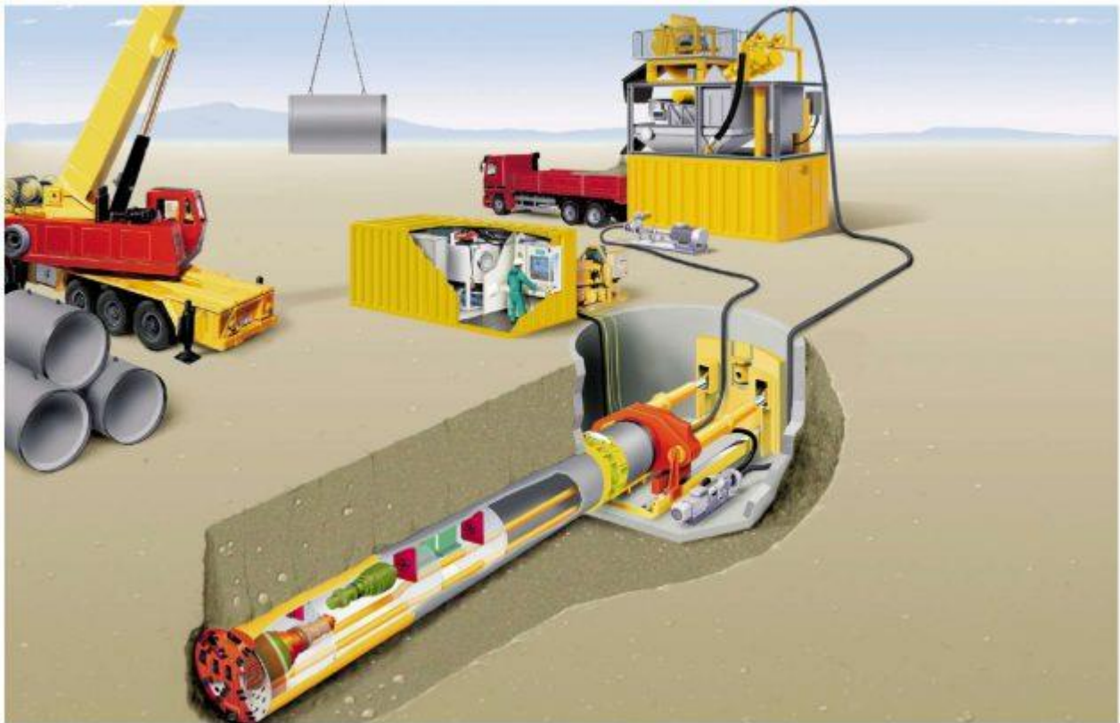
Figure 3-5 - Microtunnelling schematic showing shaft and microtunnel boring machine (image courtesy of Herrenknecht and SDL)
