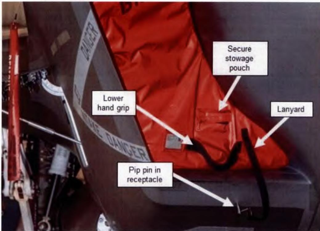
**Figure 1.4.11 – Installed intake blank showing lanyard and pip pin.**
