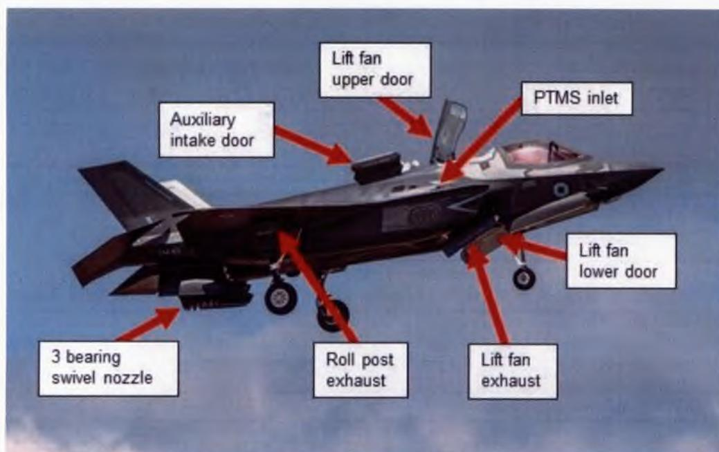
Figure 1.3.3 – F-35B in Mode 4 STOVL mode (side view).
