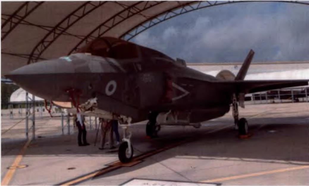
**Figure 1.3.8 – Locally acquired intake plugs in a UK F-35B at MCAS Beaufort.**
