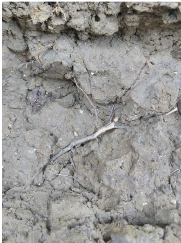
Image 4: Showing the single 4mm diameter woody root encountered at 250mm depth. A visual assessment of the root bark with hand lens suggested this root is from a hornbeam.
