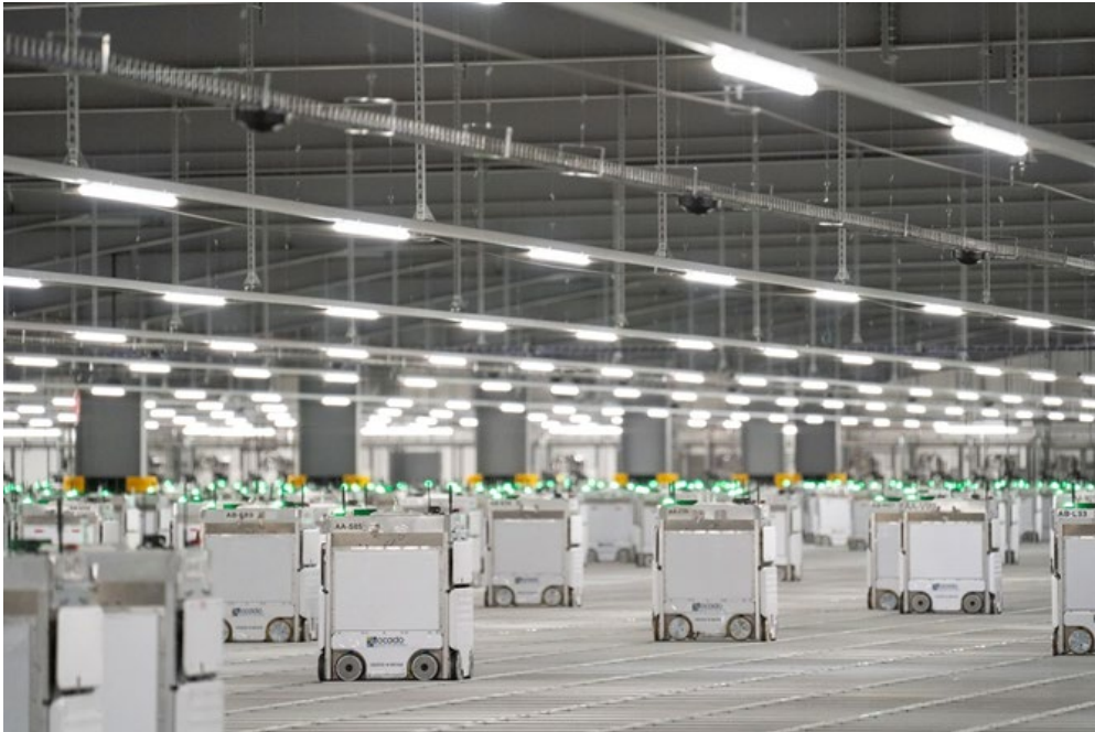
Figure 5: Robotic vehicles in use at one of Ocado's automated warehouses (© Ocado)
