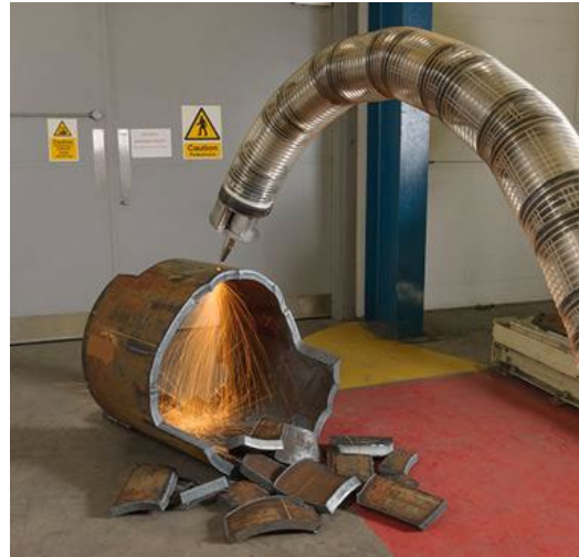
Figure 11: Laser Snake 2 – size reducing manipulator using a laser cutter (© The Welding Institute, TWI)
