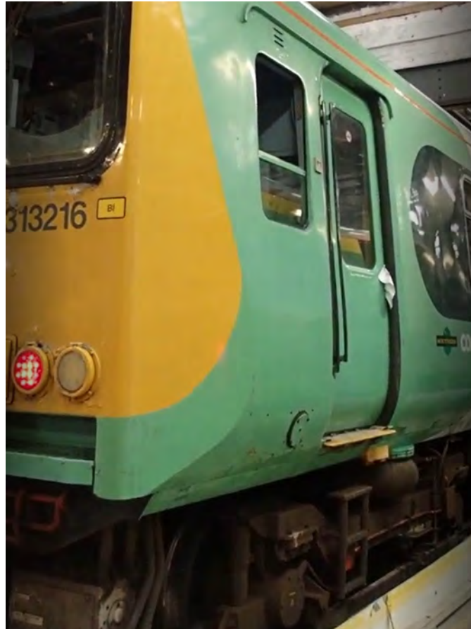
Figure 6: Image showing showing the driver's steps and handrails on train 5U57.
