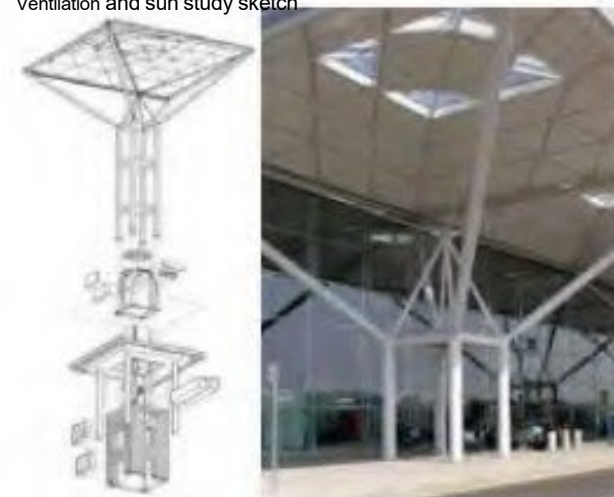
Exploded axo of structural supports
