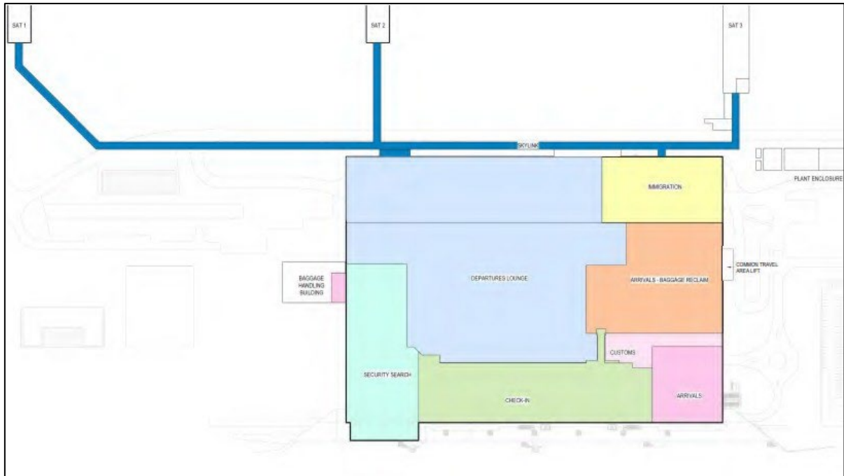
Figure 8: Plans showing the position of the proposed new three sky links to the Stansted Airport Terminal (MAG 2023)
