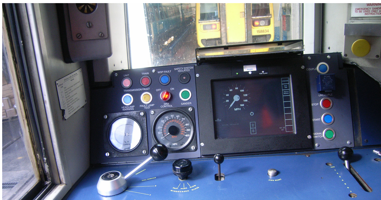
Figure 2: Typical driving cab layout and driver machine interface (DMI) screen
