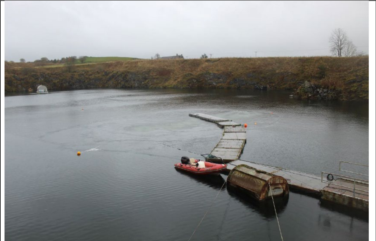
Figure 2-7 Bubble curtain with air compressor at fully output.
