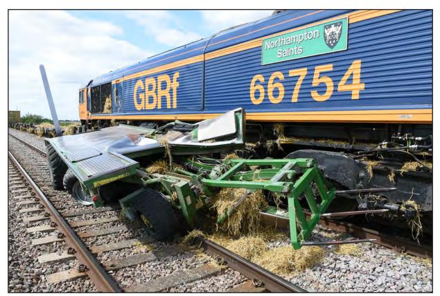
Figure 8: The bale chaser entangled with the class 66 locomotive.
