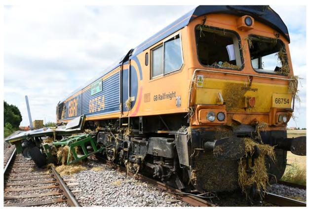
Figure 7: Damage to the front of the class 66 locomotive.
