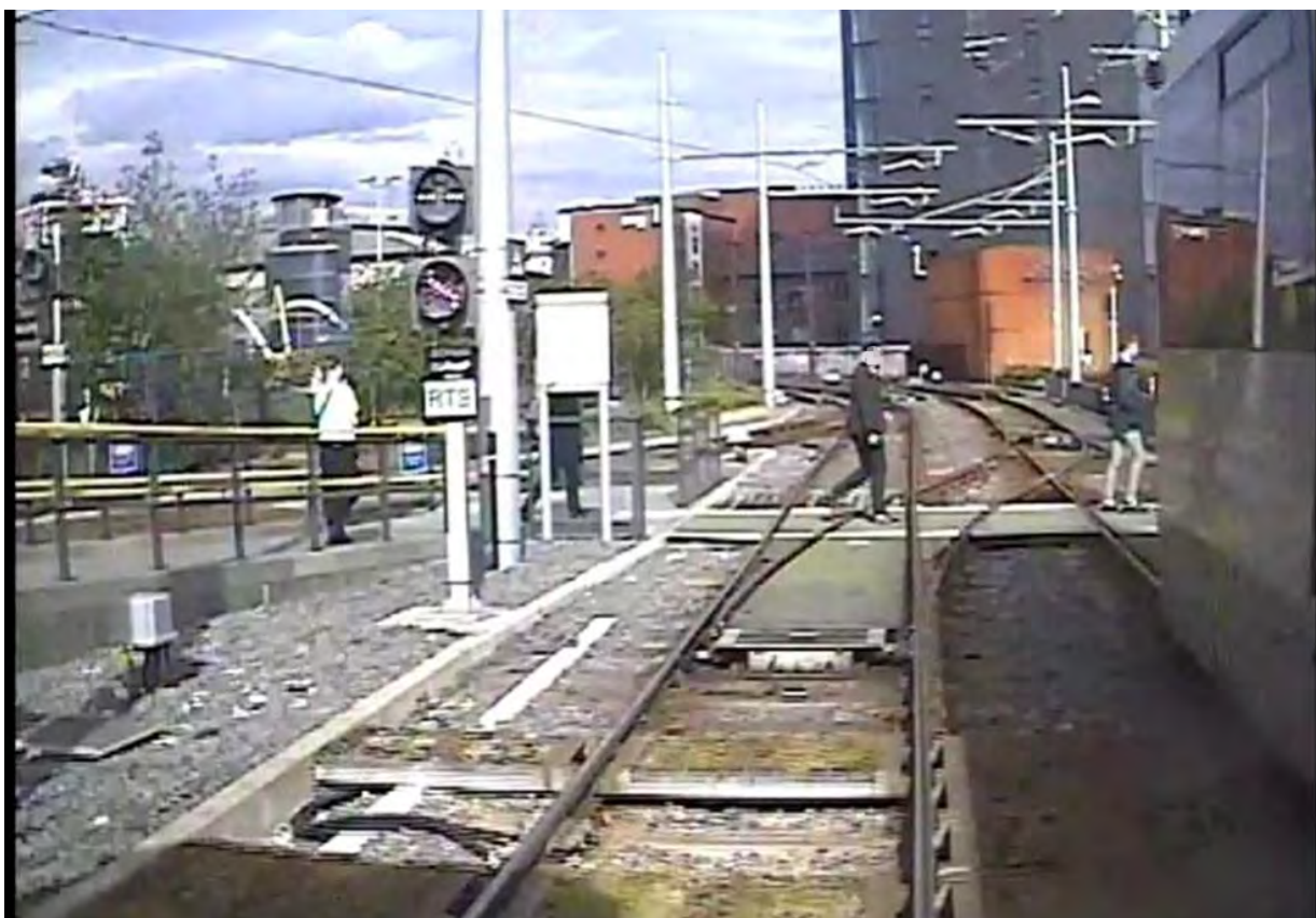
Figure 9: FFCCTV image showing signal DCF06S at STOP as tram 83 approached (image courtesy of Keolis Amey Metrolink)
