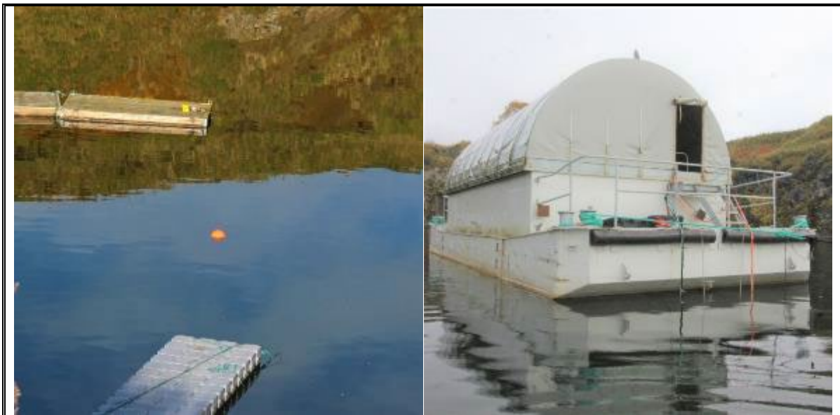
Figure 2-3 [Left] Near field pressure gauge deployment pontoons; the buoy is used to mark the position of the explosive. [Right] Far field acoustic array deployment on a floating shock test vehicle STV01.
