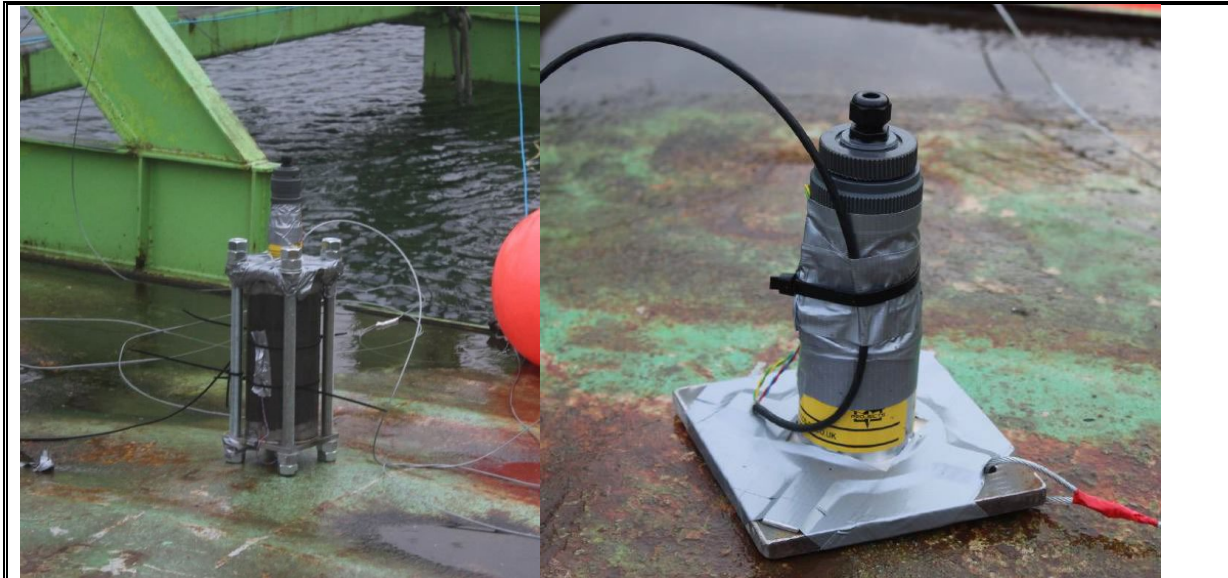
Figure 2-7 [Left] Shaped charge attached to 5kg surrogate cylinder (test 3). [Right] Close up image of the shaped charge attached to a steel plate (test 7).
