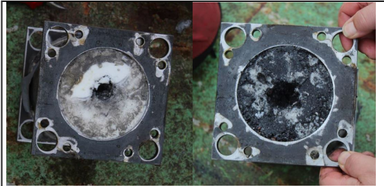
Figure 2-11 [Left ] PE4 explosive inside of 2.5 kg surrogate shell after deflagration Test 4. [Right] PE4 explosive inside of 5 kg surrogate shell after deflagration Test 6.
