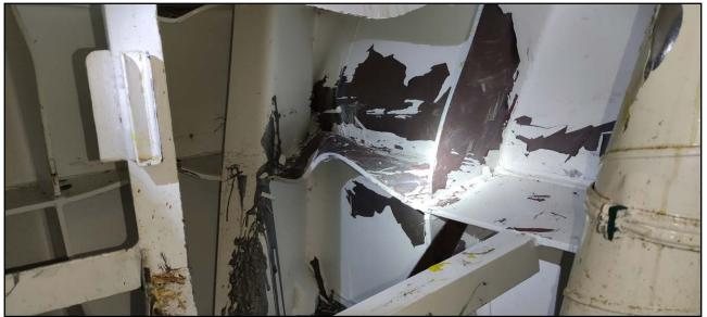
Figure 18: Damage to Scot Carrier's internal bow structure
