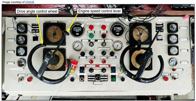
Figure 27: Karin Høj's azimuth drive controllers
