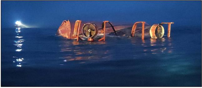
Figure 13: Karin Høj's upturned hull, showing azimuth drive units at the stern
