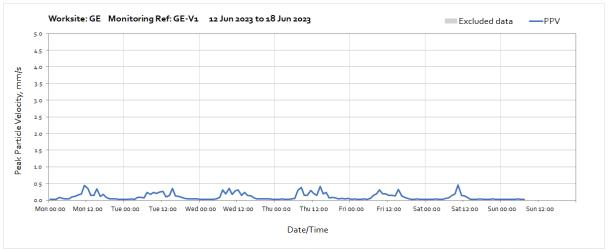
Note: Missing data from 06:00 Sunday  $18^{th}$  June until the end of the month was due to a loss of mains power to the monitor.
