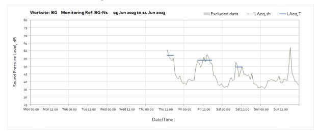
Note: Missing data for the beginning of the month was due to loss of power to the monitor caused by faulty batteries, improved replacement batteries have been installed and monitoring recommenced at 13:00 on Thursday 8<sup>th</sup> June.
