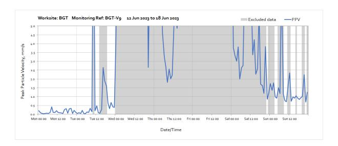
Note: High vibration levels from 10:00 to 11:00 on Tuesday 13<sup>th</sup> June was due to a field calibration. From 14:00 to 19:00 on the same day high levels occurred that have been attributed to mole activity. High vibration levels due to mole activity occurred from 15<sup>th</sup> June onwards.
