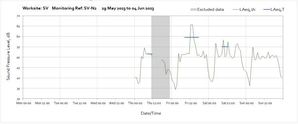
Note: Partially missing data from 11:00 on Thursday 1<sup>st</sup> June to 23:00 on Thursday 1<sup>st</sup> June was due to monitor failure because of water in the case protecting the meter.
