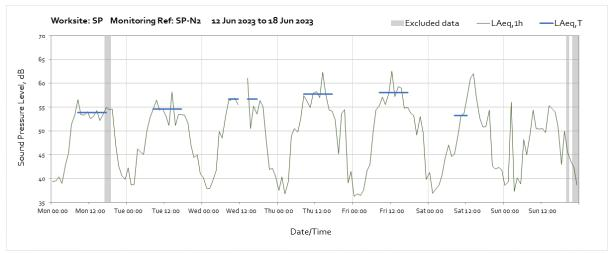
Note: Missing data from 12:00 on Wednesday 14<sup>th</sup> June to 14:00 on Wednesday 14<sup>th</sup> June was due to the meter being exchanged for calibration.
