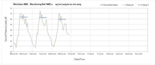
Note: Missing data from 22:00 on Wednesday 7<sup>th</sup> June until the end of the month was due to loss of power to the monitor due to solar panels being blocked by overgrown vegetation.
