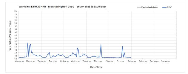
Note: High levels of vibration caused by works close to the monitor. Lower vibration levels anticipated at nearest receptor. OFFICIAL
