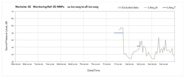
Note: Missing data from the start of the month until 13:00 on Friday 15<sup>th</sup> June was due to a damaged power cable which has now been replaced.
