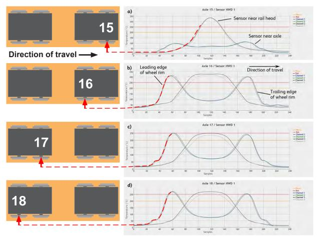
Figure 30: Recorded temperature curves from Pembrey HABD for train 6A11 on 26 August 2020, for the third wagon (axles 15 to 18). The curves for axle 15 (leading) are characteristic of a locked axle, while the curves for the other axles (16 to 18) show evidence of dragging brakes, in that high temperatures are recorded for the whole wheel, not just the tread (graphs courtesy of Network Rail)
