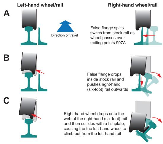
Figure 16: Diagram showing the sequence of the derailment of wagon GERS 89005
