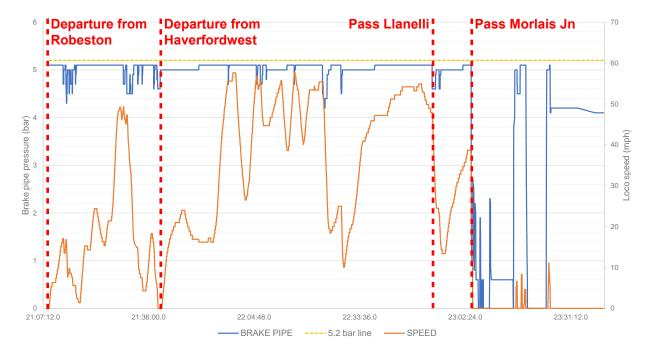
Figure 8: Data recorded by the on-train data recorder (OTDR) fitted to the locomotive of train 6A11 for the journey from Robeston to Morlais Junction, including the brake pipe pressure (blue solid line), 5.2 bar pressure line (yellow dotted line), speed (orange solid line) and locations en route
