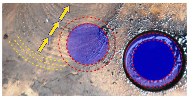
Figure 22: Microscopic image showing the original location and a surface imprint on the mating face of the relay valve (red dotted lines) of what is believed to be an undamaged load sensing device 'O' ring. Also shown to the left (yellow dotted lines and arrows) are surface imprints of the same 'O' ring as it migrated up towards the auxiliary reservoir and brake cylinder ports (see figure 23)
