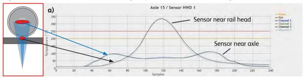
Figure 29: Diagram (left) showing the locations of the HABD sensors in relation to measurements taken from the axle box area of a wagon (shown as channels 1 and 2) and contact point between a wheel and the rail (channels 3 and 4). The graph (right) shows the temperature curves for the locked wheel of train 6A11 (Diagrams courtesy of Network Rail)
