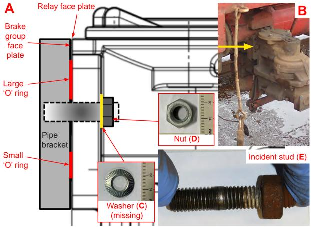
Figure 24: Diagram (A) showing the position of the stud, nut and missing washer with inset image (B) showing the location of the mating faceplates. A washer (C), and nut (D) compared to one of two incident studs (E) attached (through corrosion) to the nut.
