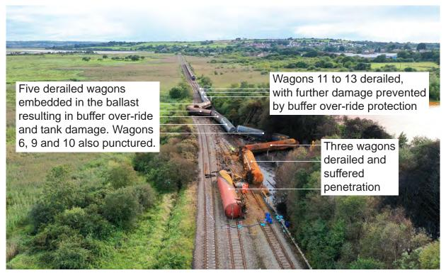
Figure 18: Aerial image of the accident site looking towards the rear of train 6A11(image courtesy of South Wales Fire and Rescue)
