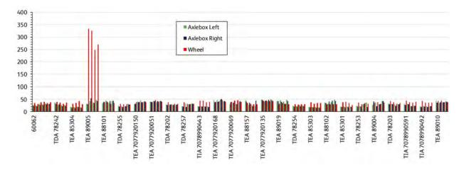
Figure 28: HABD data for train 6A11 showing temperatures recorded for all wagons
