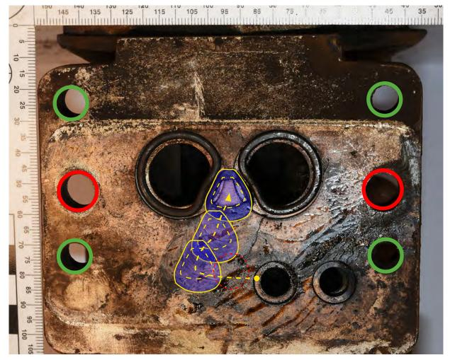
Figure 23: The relay valve mating face and what is believed to be the path taken by the variable load sensing device 'O' ring (yellow dashed line). Pre-1994 design incorporated four fixing points (green circles) and later design change to two fixing points (red circles)
