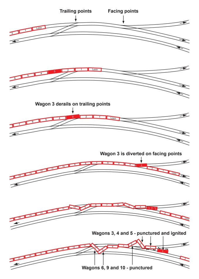
Figure 15: Diagram (from top to bottom) showing the likely sequence of the train derailment
