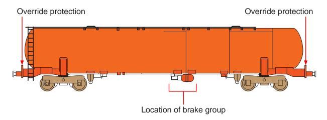
Figure 9: Diagram of a GF4-SS1 brake group on a GERS TEA type wagon
