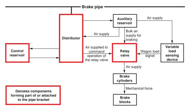
Figure 10: Schematic diagram of the wagon braking system showing the relationship between the various components including the distributor, control reservoir, auxiliary reservoir, relay valve, variable load sensing device, brake cylinders and brake blocks
