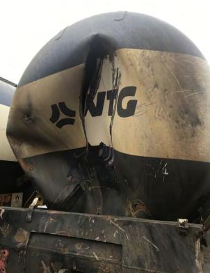
Figure 31: (left) VTG wagon (incident wagon 7) with raised buffer override protection beams which mitigated against further damage occurring and (right) wagon (incident wagon 6) that derailed, showing impact damage at high level where override protection could not prevent override and puncturing.
