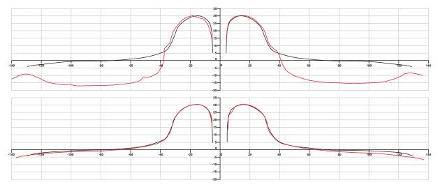
Figure 14: Diagrams showing the left (LHS) and right (RHS) wheel profiles (shown as black line) on the front axle (top) and rear axles (bottom) of wagon GERS 89005. The front axle (also shown as axle 15 on the HABD data on figure 29) also shows the depth (shown as a red line) of wear on the tread of the locked wheels. The treads on the rear axles (also shown as axles 16 to 18 on figure 29) show a lower depth of wear as these wheels were not locked although the brakes were dragging
