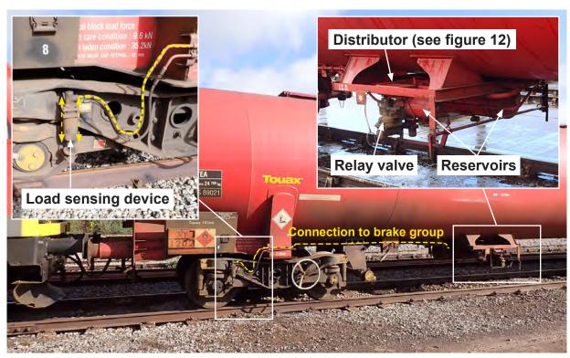
Figure 11: GF4-SS1 brake group on a TEA type wagon
