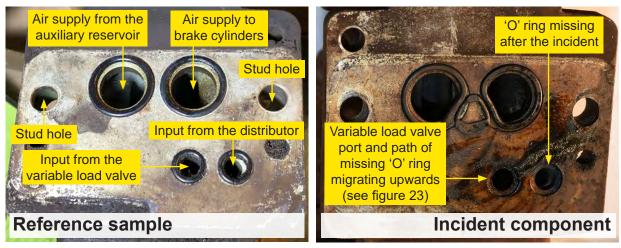
Figure 21: Image showing the correct 'O' ring locations of a refence sample (GERS 89014) in comparison to the incident wagon (GERS 89005)
