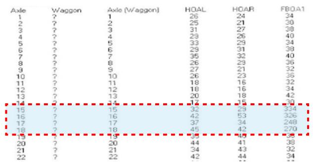
Figure 27: Diagram of the HABD data provided for train 6A11 on 26 August showing axles numbers 1 (front) to 4 (rear) for wagon GERS 89005 (labelled 15 to 18), with corresponding temperatures shown in degrees Celsius
