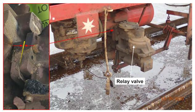
Figure 12: Image (main) showing the connection between the pipe bracket and the relay on a GF4-SS1 brake group with inset image showing the 1-2 mm gap (yellow segment) found between the pipe bracket and the relay valve on wagon GERS 89005
