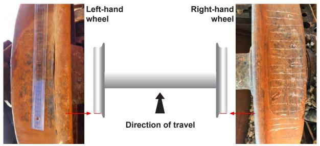
Figure 13: Images showing the profile of the wheel and the damage (red line) that occurred to the left and right wheels on the leading axle of wagon GERS 89005
