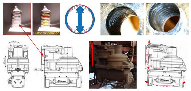
Figure 25: Images (top right and middle) showing the damaged surfaces of the internal bores of the mounting holes of the relay valve (bottom image and diagrams) as a result of the relay valve being loose and pivoting on the studs of the brake group. The inset image (top left) shows the castings taken from the bores for analysis of the marks which confirm that the relay was loose.
