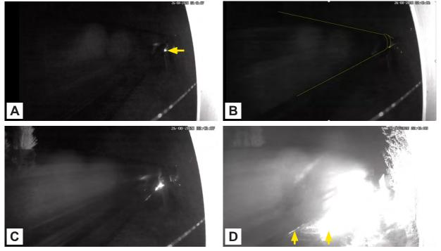
Figure 6: CCTV images ((a) to (d)) showing train 6A11 and wagon GERS 89005 passing Pen-y-bedd AHBC showing sparks emanating from the left and right wheels on the front wheelset
