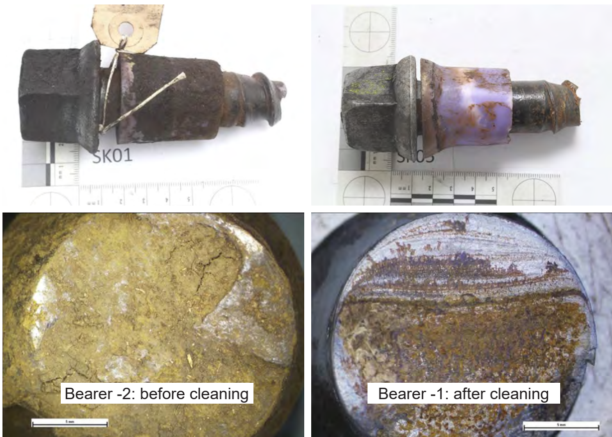
Figure 15: Examples of broken track screws, showing fracture surfaces during examination
