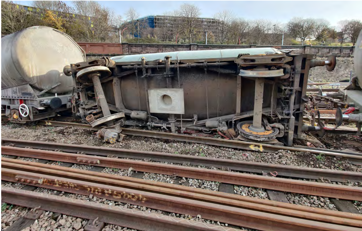
Figure 3: Wagon BCC10756 toppled on its side
