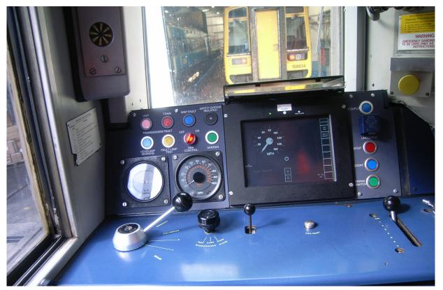
Figure 2: Typical driving cab layout and driver machine interface (DMI) screen
