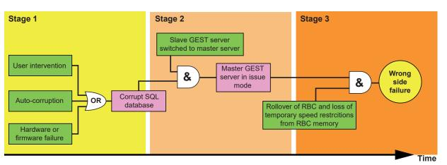
Figure C6: Sequence of events from SQL database corruption to loss of temporary speed restrictions
