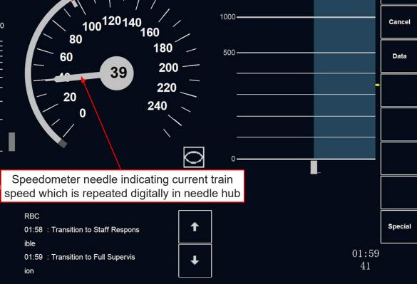
Figure 3: DMI screen showing speedometer with maximum speed supervision and actual speed
