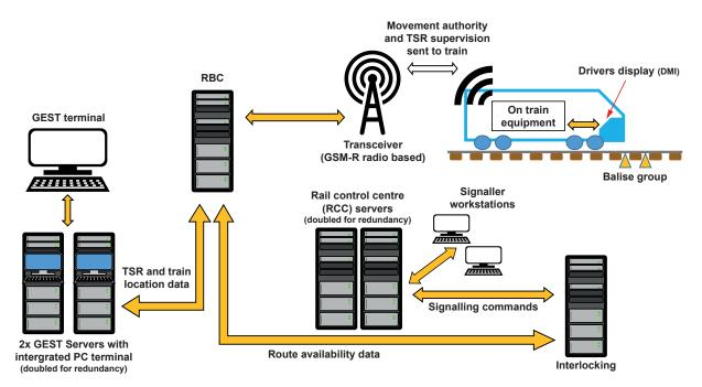
*Figure 7: Simplified diagram of Cambrian ERTMS showing sub-systems relevant to the investigation. Note, SILAM / SICAM sub-system not shown.*
