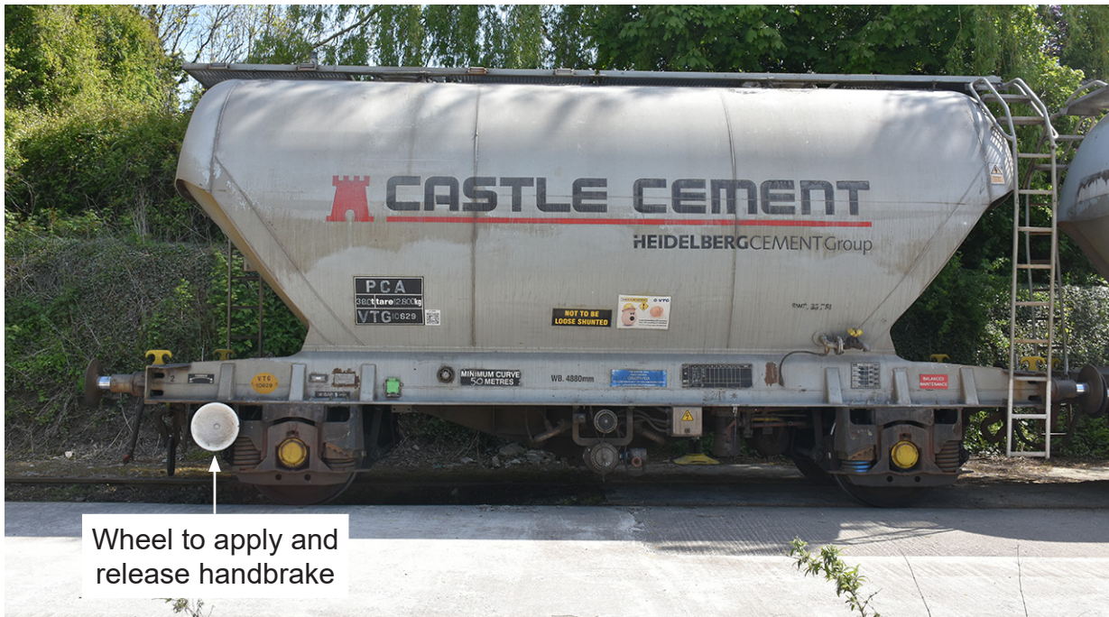
Figure 7: An example of a PCA tank wagon
