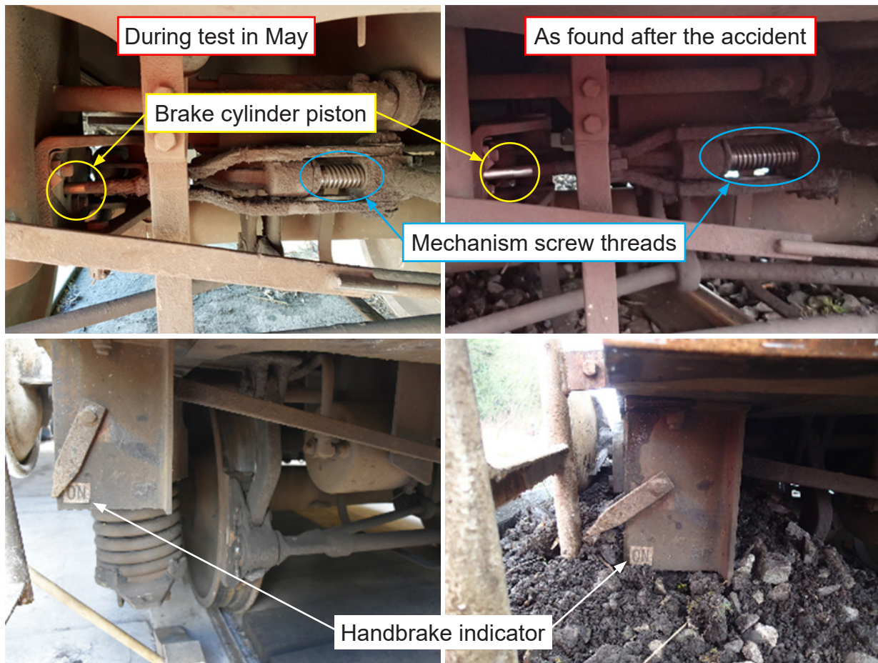
Figure 14: Comparison of the positions of the handbrake components during testing and as found after the accident
