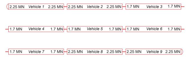
Figure 17: Distribution of coupler collapsing strength along the IET rake
