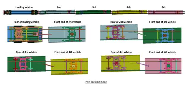
Figure 14: Output from collision and derailment simulation – bird's eye view (courtesy of Hitachi)
