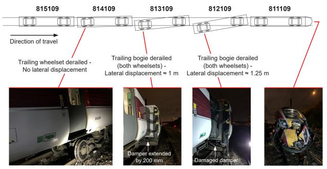
Figure 9: Schematic showing extent of derailment during collision (not to scale)
