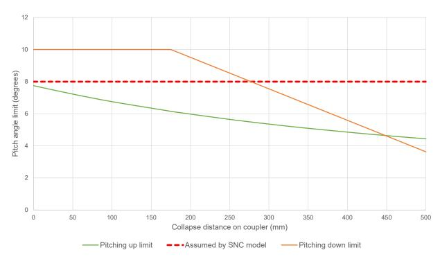
Figure 12: Graph showing how the pitch limits change as the inter-vehicle coupler collapses<sup>12</sup>
