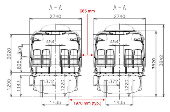
Figure 10: Typical passing clearance between two IETs on adjacent tracks
