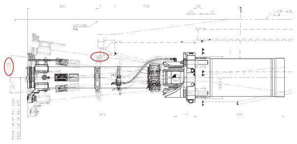
Figure 11: Coupler pitch up movement and limit due to coupler contacting the carbody (courtesy of Hitachi)
