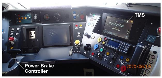
Figure 4: Class 800 cab layout showing TMS and power brake controller
