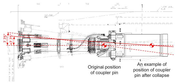
Figure 16: Effect of coupler collapse on pitch freedom
