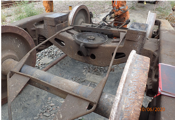
Figure 36: The 1-4 end bogie and bogie centre pivot after removal from wagon 3415
