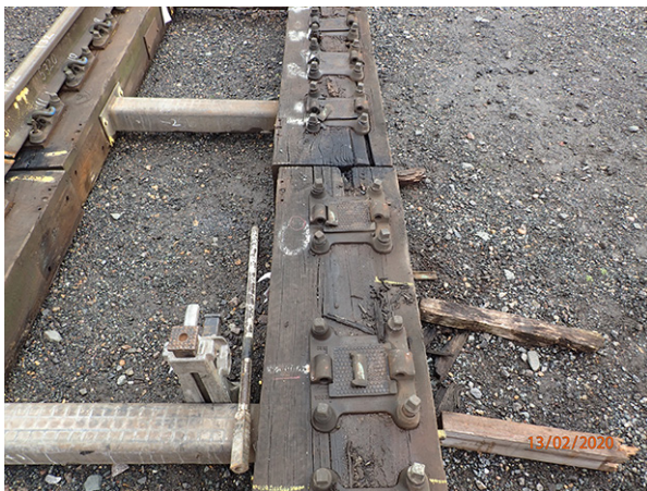
Figure 16: Longitudinal timbers laid out for examination following removal of the right-hand (six-foot) rail. Timber 2L is nearest the camera with 1L beyond it.
