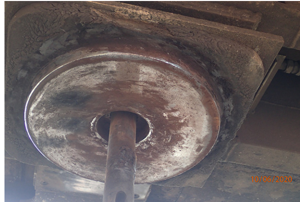
Figure 37: The 2-3 end top centre pivot with pin, located on the underside of the wagon's underframe
