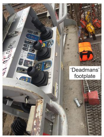
Figure 8: The control console and 'deadmans' foot control on MEWP 10
