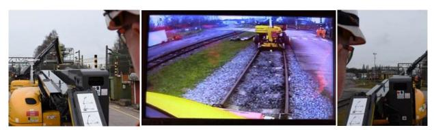
Figure 11: Images taken from MEWP 10, 15 metres from stationary MEWP 3, showing the view from the machine operator's eye level (left), CCTV monitor view (middle) and machine operator eye level view (right) from MEWP 10
