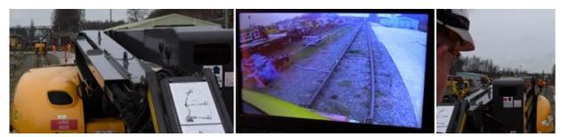
Figure 10: Images taken from MEWP 10, 107 metres from stationary MEWP 3, showing the view from the basket (left), CCTV monitor view (middle) and eye level view (right) from the machine operator's perspective on MEWP 10
