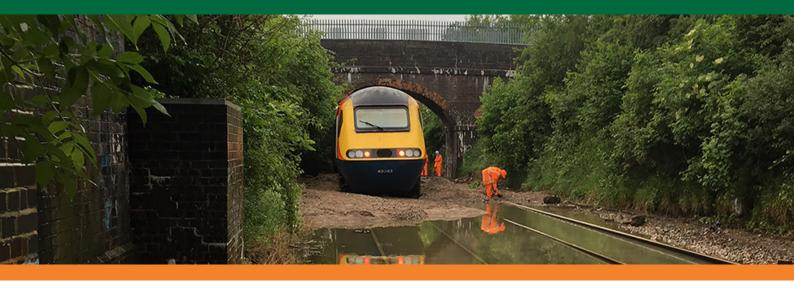
Train collision with material washed out from a cutting slope at Corby, Northamptonshire 13 June 2019
