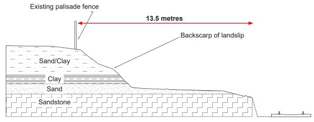
Figure 17: The geology of the failed cutting slope
