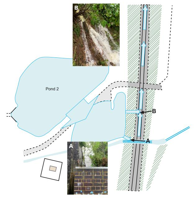
Figure 9: The flow of water from pond 2, through the field and onto the railway. Inset image A shows flood water flowing down the stepped flume on the northern side of the aqueduct. Inset image B shows flood water flowing onto the railway at the foot of the cutting slope.
