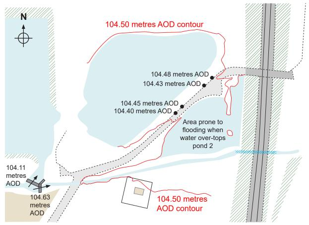
Figure 14: The levels as recorded by the surveys for the spillways and ground showing the low point on the eastern bank of pond 2
