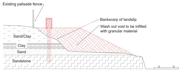
Figure 26: Drawing of Network Rail's repair to the cutting slope
