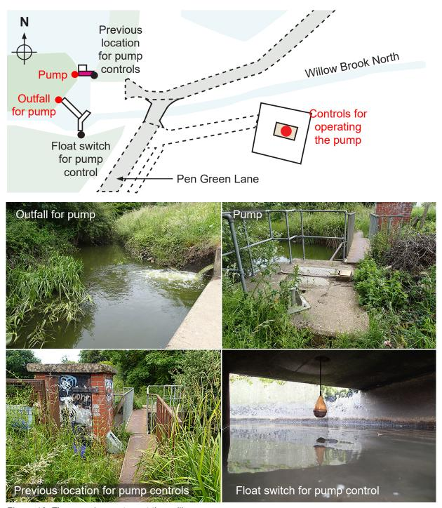
Figure 16: The pumping system at the spillways
