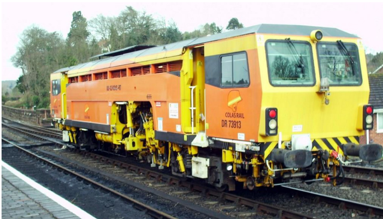
Figure 4: The tamper involved in the incident (courtesy of Colas Rail)
