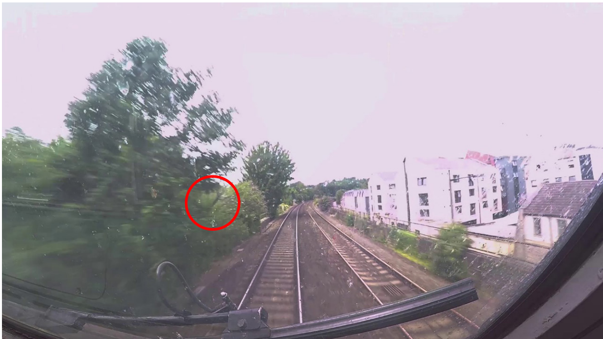
Figure 4: Forward Facing CCTV from July 2018, showing tree amongst growing vegetation (courtesy of Network Rail)
