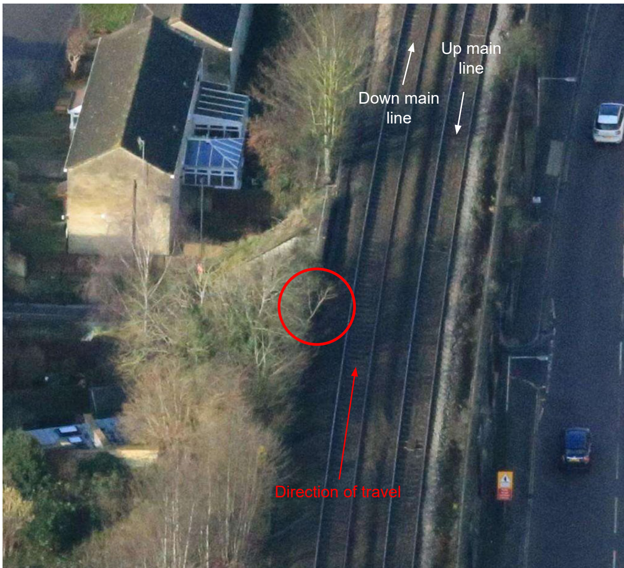
Figure 2: General photograph of the scene before the accident showing the tree branch involved (circled) (courtesy of Network Rail)
