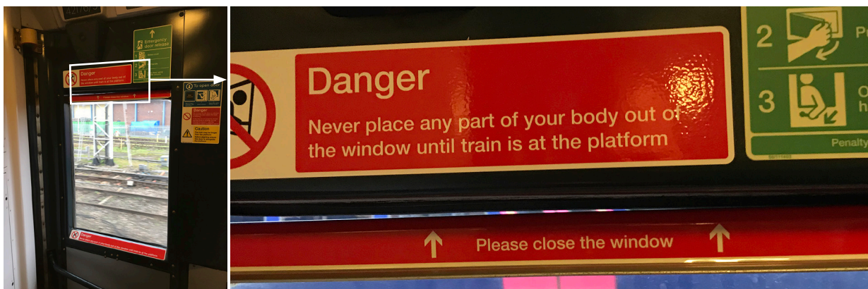
Figure 8: Photograph showing revised signage as fitted by GWR
