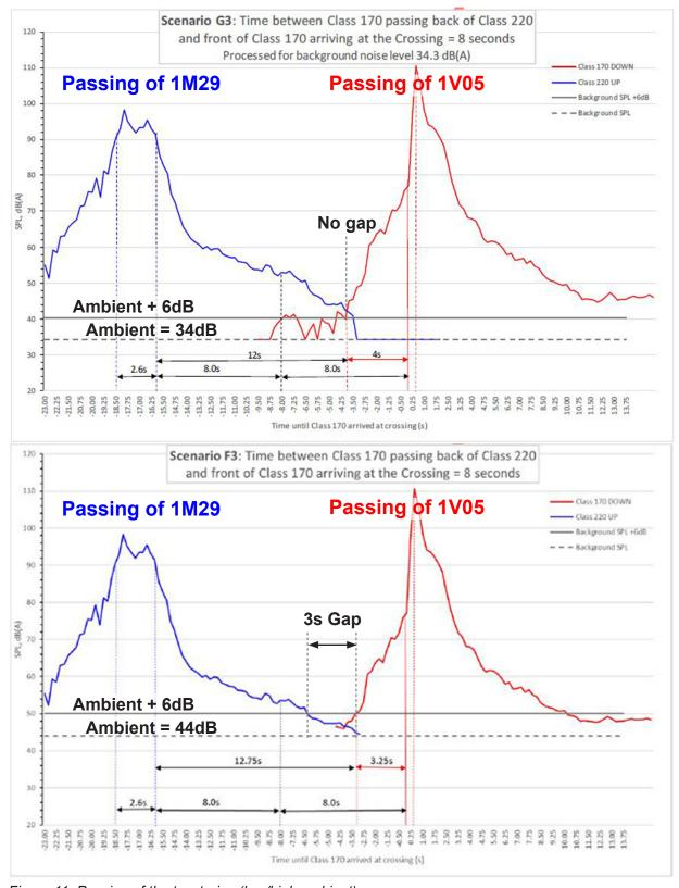
Figure 11: Passing of the two trains (low/high ambient)
