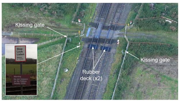
Figure 4: Layout of Tibberton No. 8 footpath crossing (image courtesy of Network Rail)
