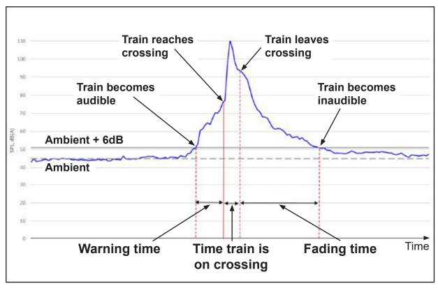
Figure 10: Typical sound trace recorded at Tibberton No. 8 footpath crossing
