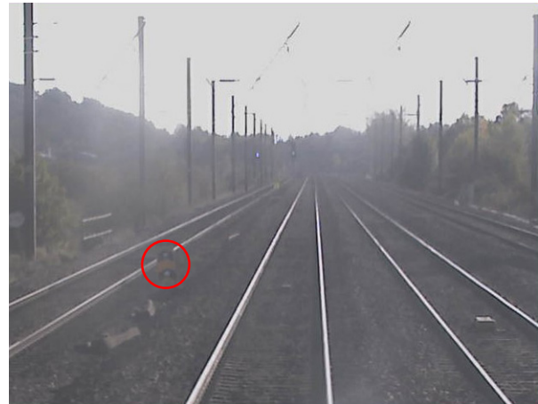
Figure 7d: FFCCTV view of ESI board about a second away from it (image courtesy of LNER)
