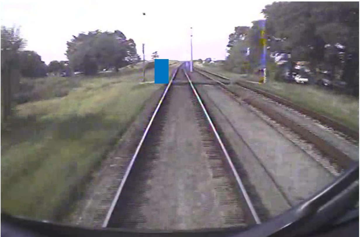
Figure 5: Edited image from the FFCCTV of tram 260 at around 18 metres from the crossing and 1.2 seconds before the collision. The rectangle indicates the location of the pedestrian.
