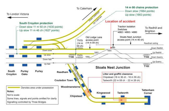
Figure 2: Line diagram showing Stoats Nest Junction and other key locations
