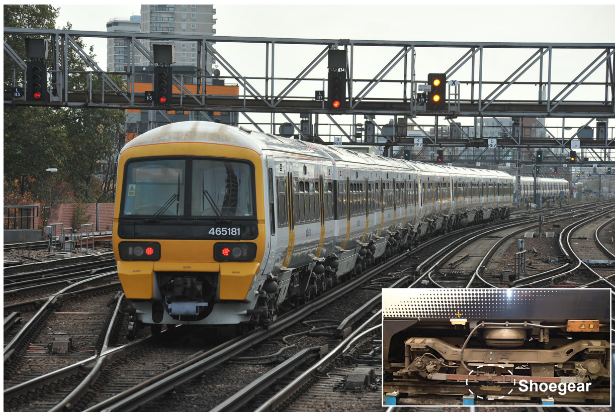
Figure 5: Typical Southeastern Networker class 465 electric multiple unit. Inset shows the shoegear equipment. (Main image courtesy of London and South East Railway Ltd.)
