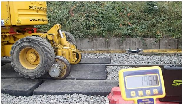
Figure 16: Pull-test when road wheels acting only (DRWB callipers removed)
