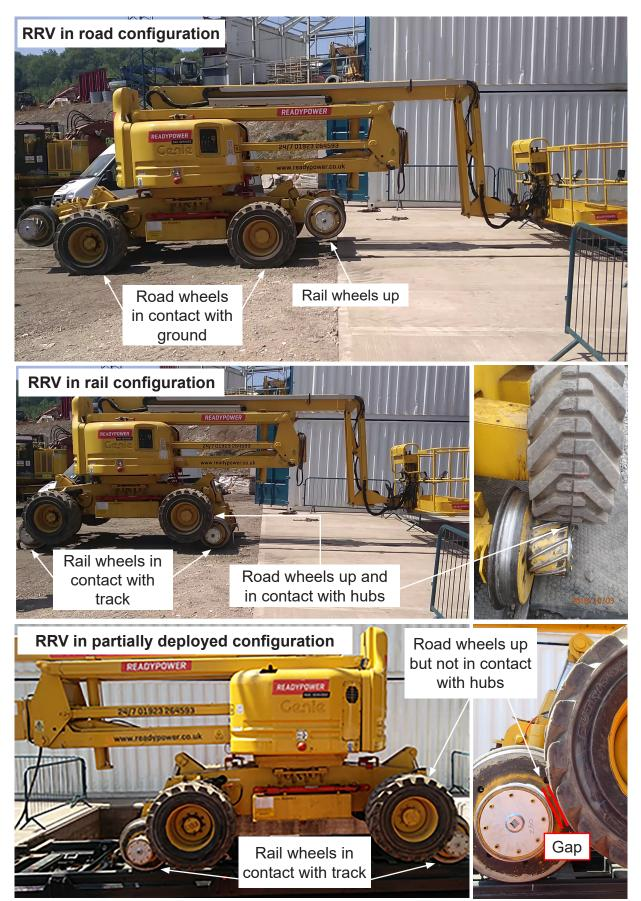
Figure 5: RRV in various deployment configurations
