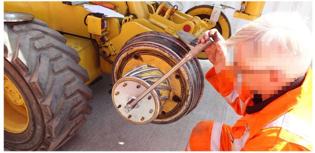
Figure 15: Torque testing of DRWB system
