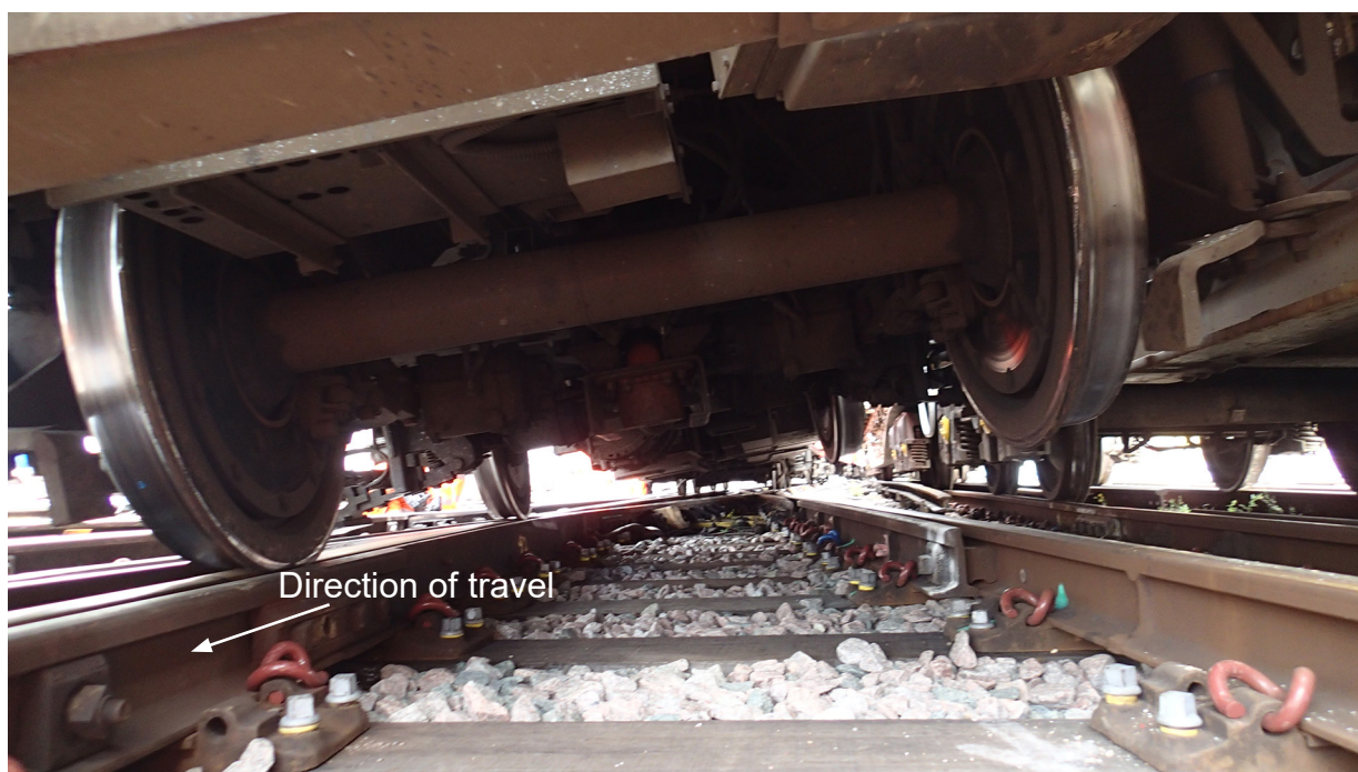
Figure 9: Train 2D03 with left (in direction of travel) wheels of the leading bogie above the rail
