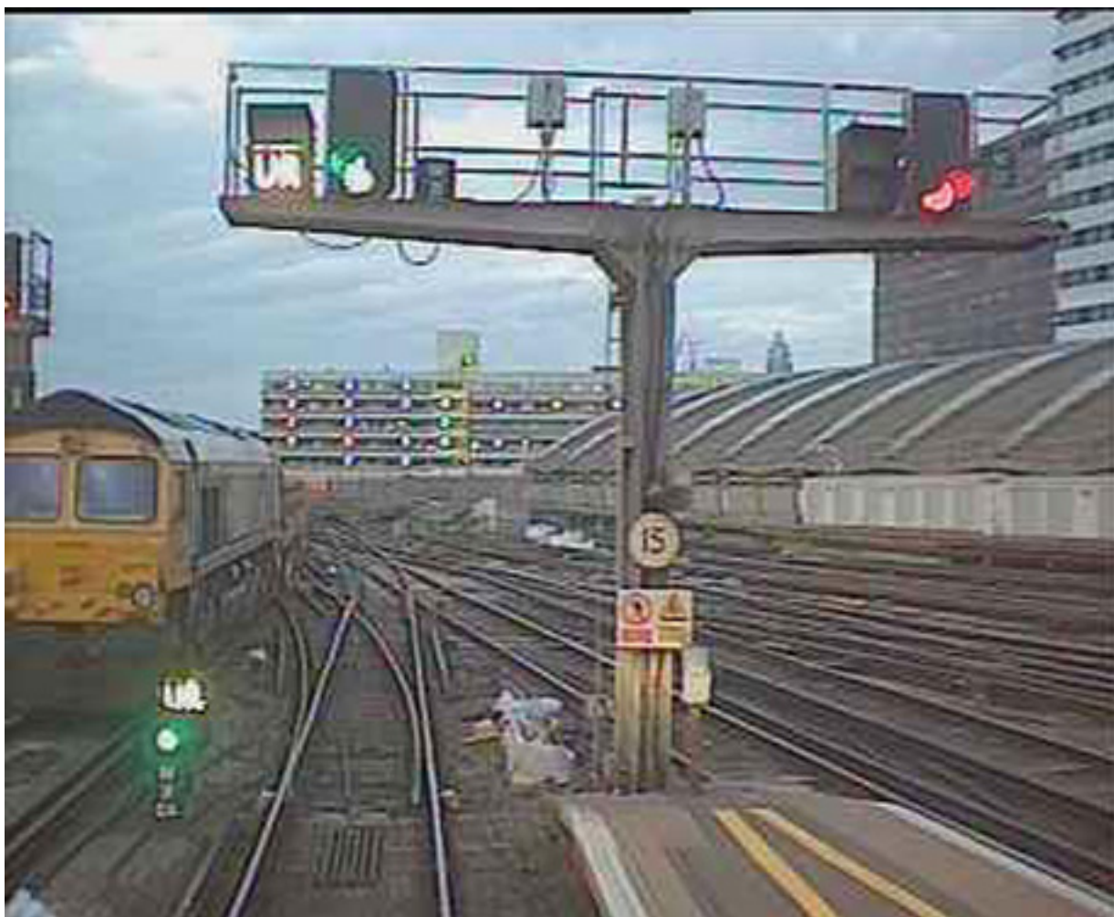
Figure 7: Forward facing CCTV from train 2D03 showing the green signal and 'UR' (up main relief) route indication displayed at high and low levels as it departed from platform 11 (courtesy South Western Railway)
