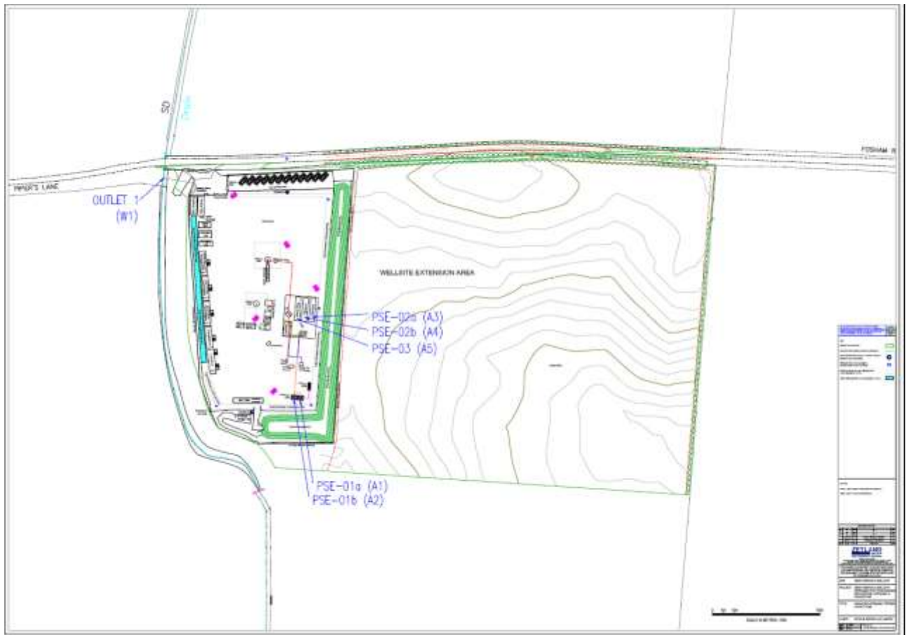
Figure 2: Indicative layout – appraisal/ testing layout with air emission points (PSE)
