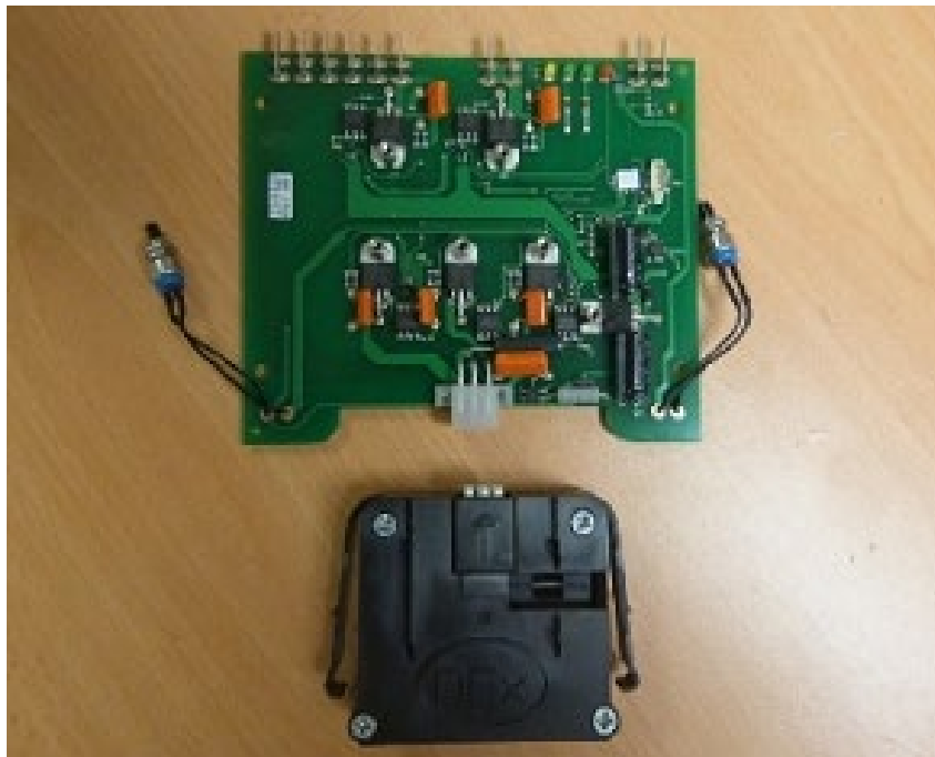
Figure 16 - DFX replacement plug and circuit board
