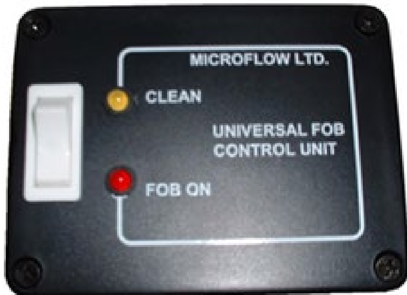
Figure 20 - Alternative FOB monitor switch box
