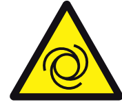
Machinery starts automatically
