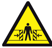
Danger of entrapment
