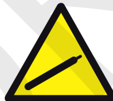
Danger Compressed gas
