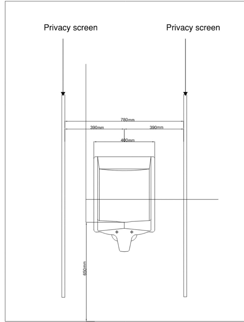
**Figure 32: Indicative diagram showing urinal placement and setting out (plan and elevation).**
