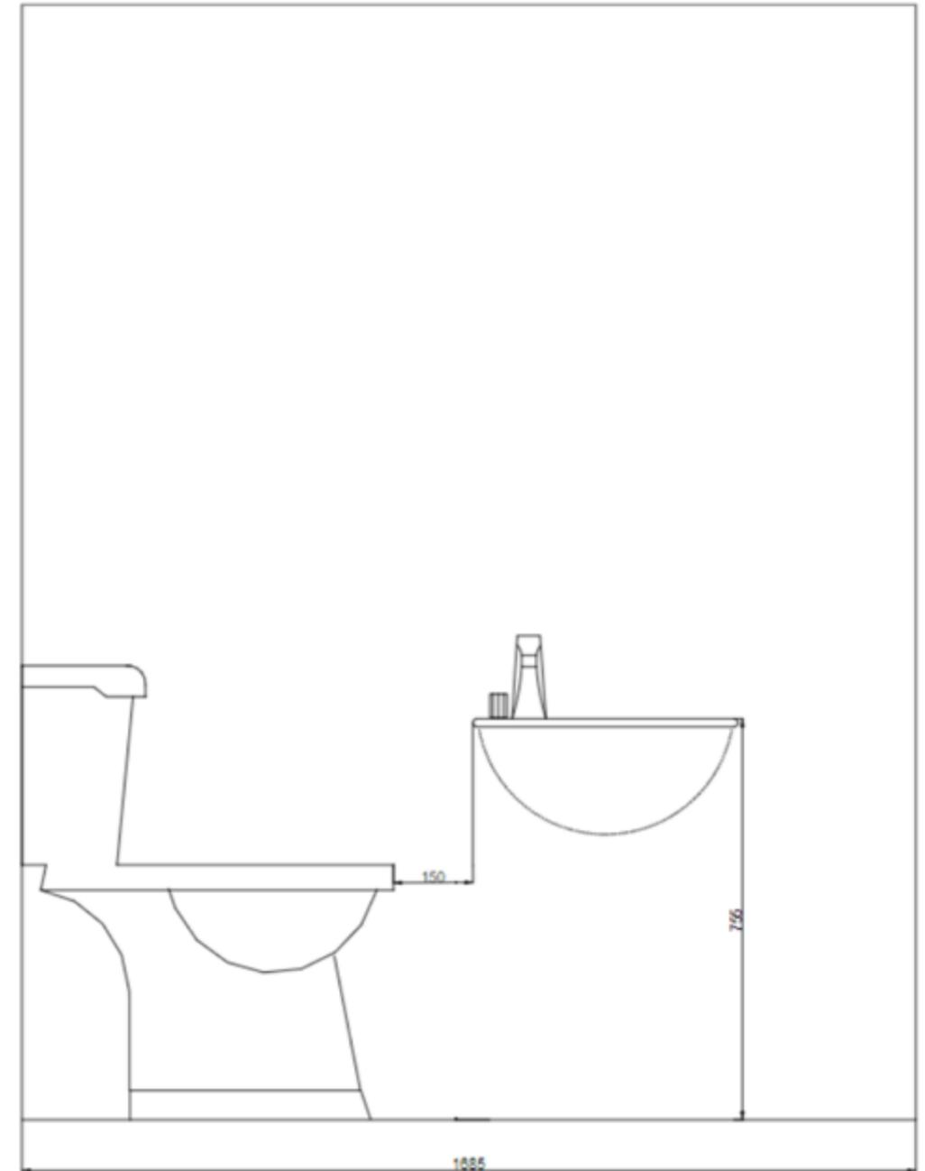
Figure 29: Indicative diagram for standard toilet cubicle with basin (plan and elevation).
