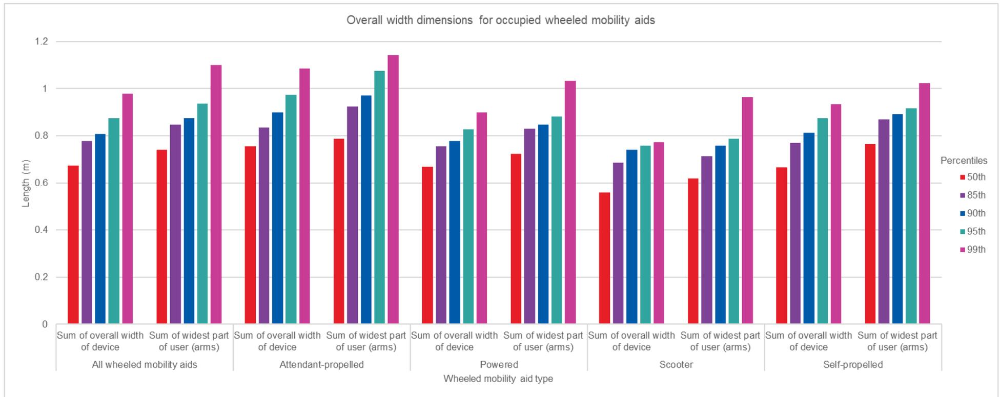
**Figure 8. Key dimensions for occupied wheeled mobility aids – by type of wheeled mobility aid.**
