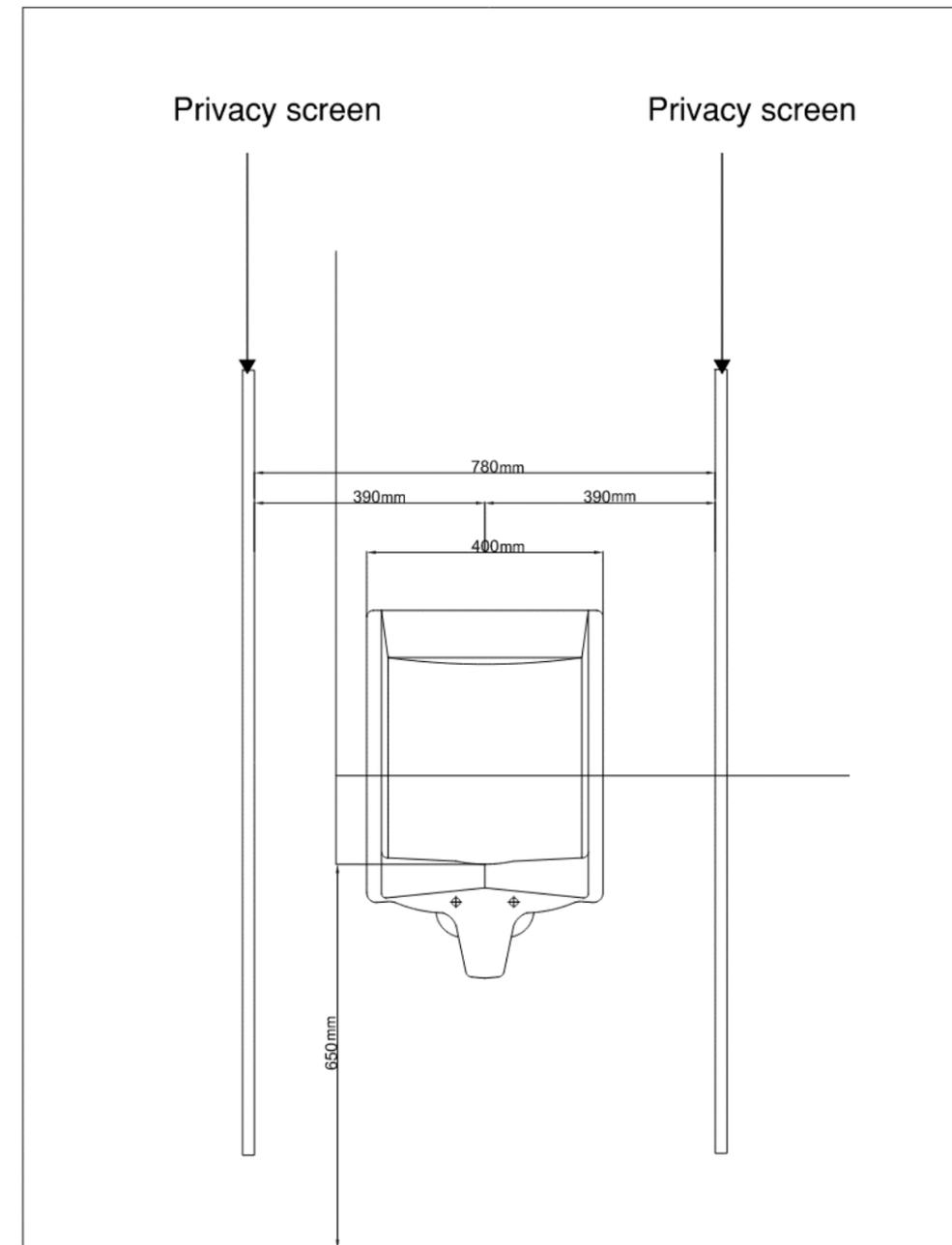
**Figure 32: Indicative diagram showing urinal placement and setting out (plan and elevation).**
