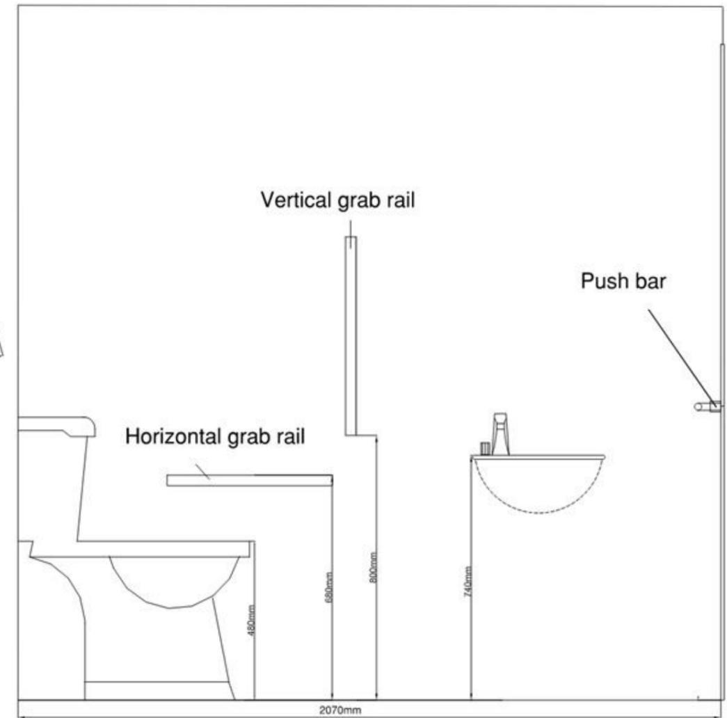
**Figure 30. Indicative diagram for ambulant accessible toilet cubicle with basin.**
