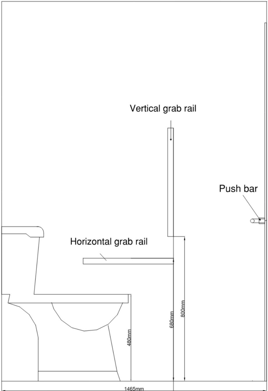
Figure 33: Indicative drawing for toilet for ambulant disabled people (without a basin) (plan and elevation).
