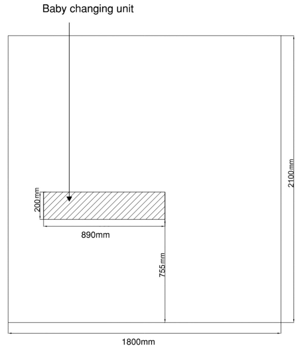
**Figure 35: Indicative drawing for a toilet with baby changing facilities and space for a CTD (elevations).**
