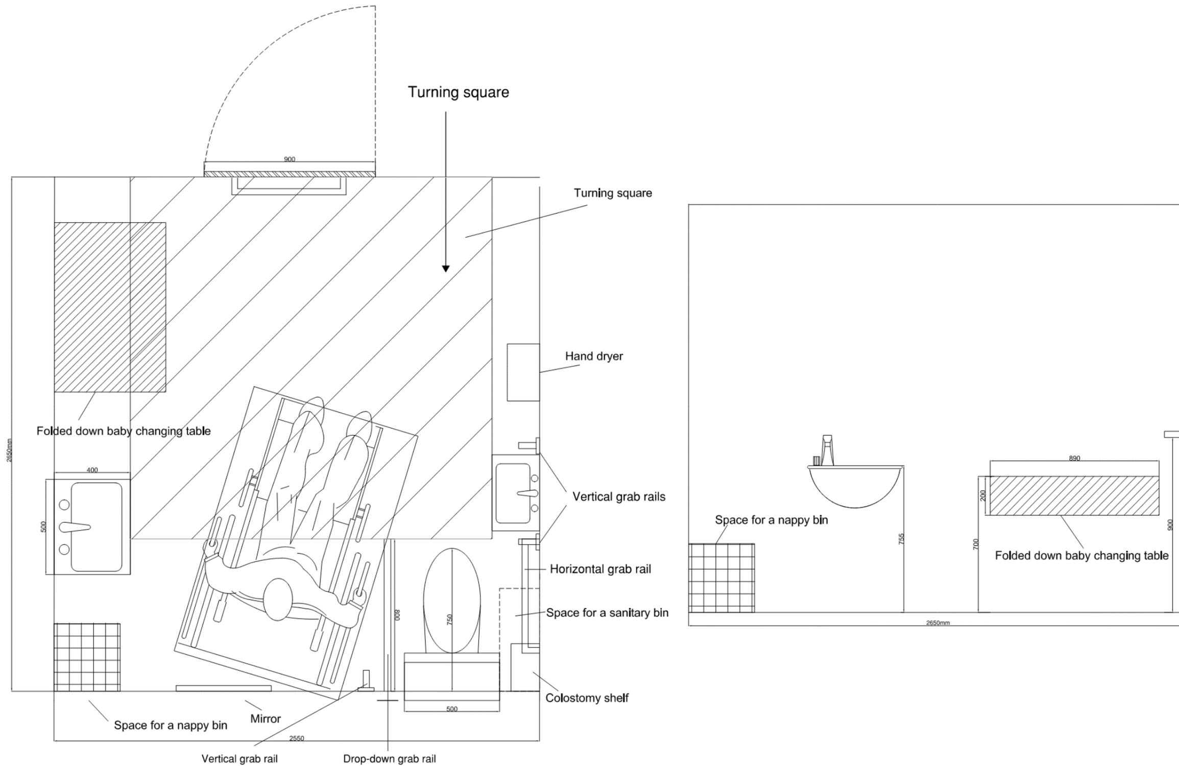
**Figure 37: Indicative drawings for a wheelchair-accessible toilet with baby changing facilities (plan and elevation)**
