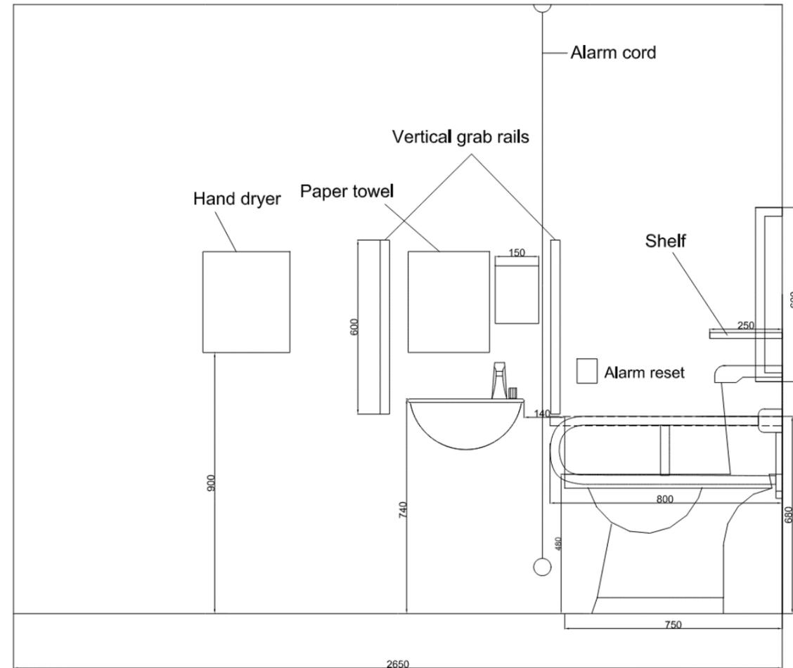
**Figure 36: Indicative drawing for a wheelchair-accessible toilet facility for independent use (plan and elevation)**
