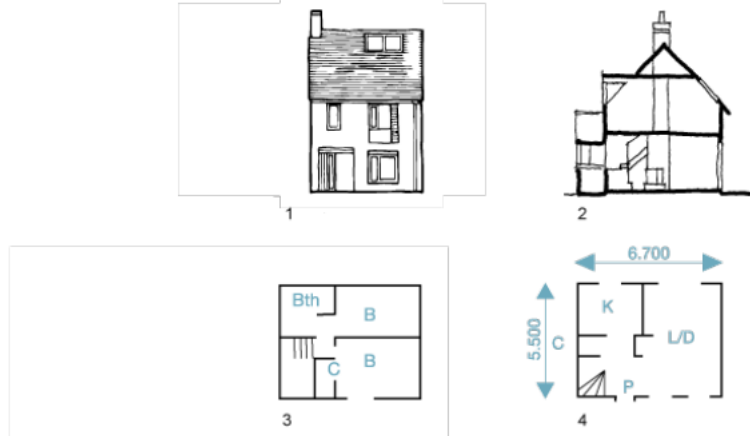
1. Front elevation 2. Section 3. First-floor 4. Ground-floor
