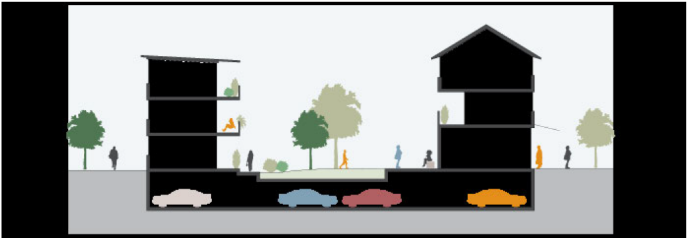
Underground parking with communal space above
