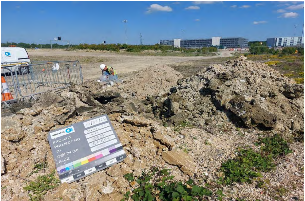
TP04 GL to 4.00m Spoil
