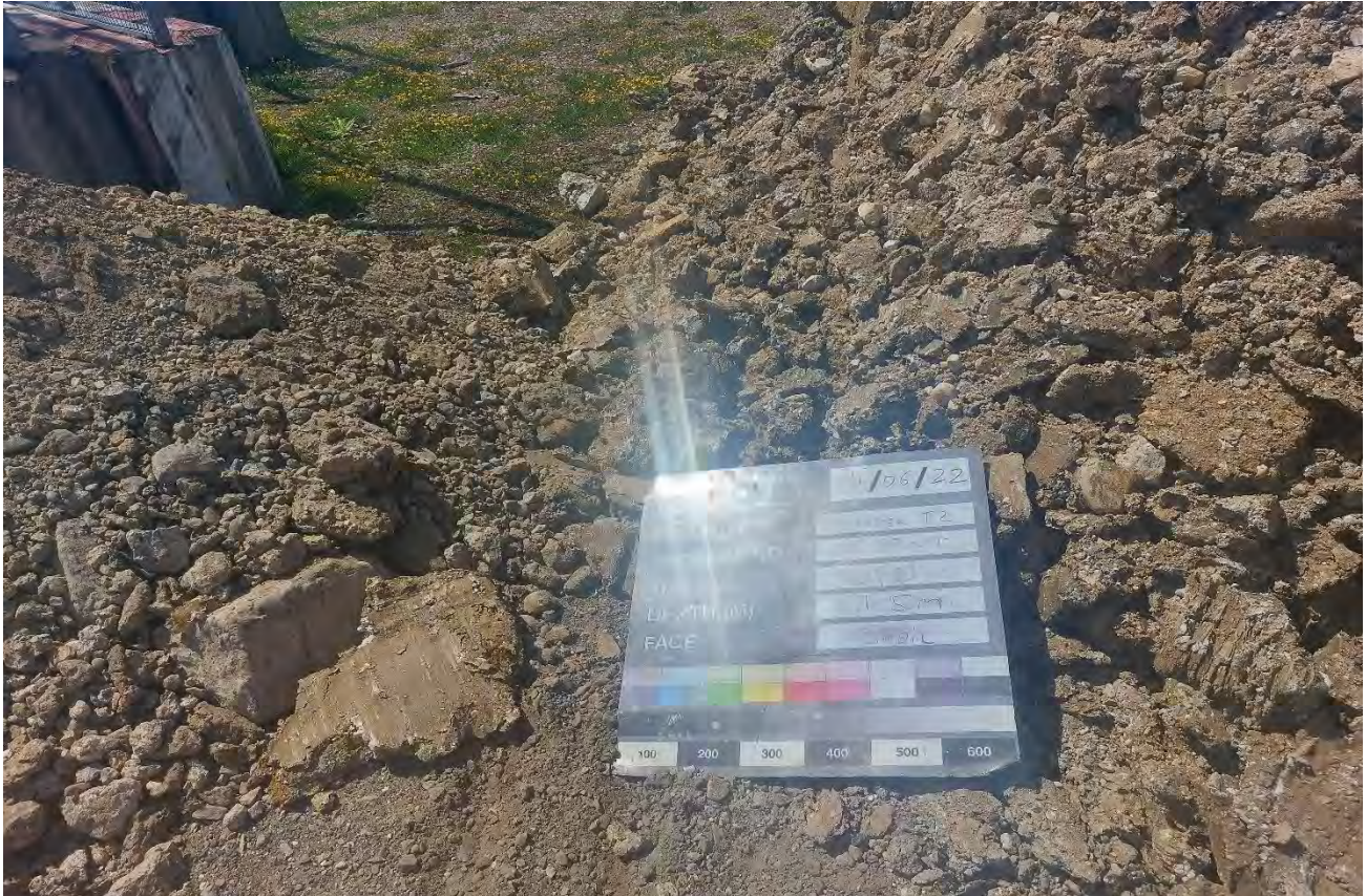
TP01 GL to 4.00m Spoil
