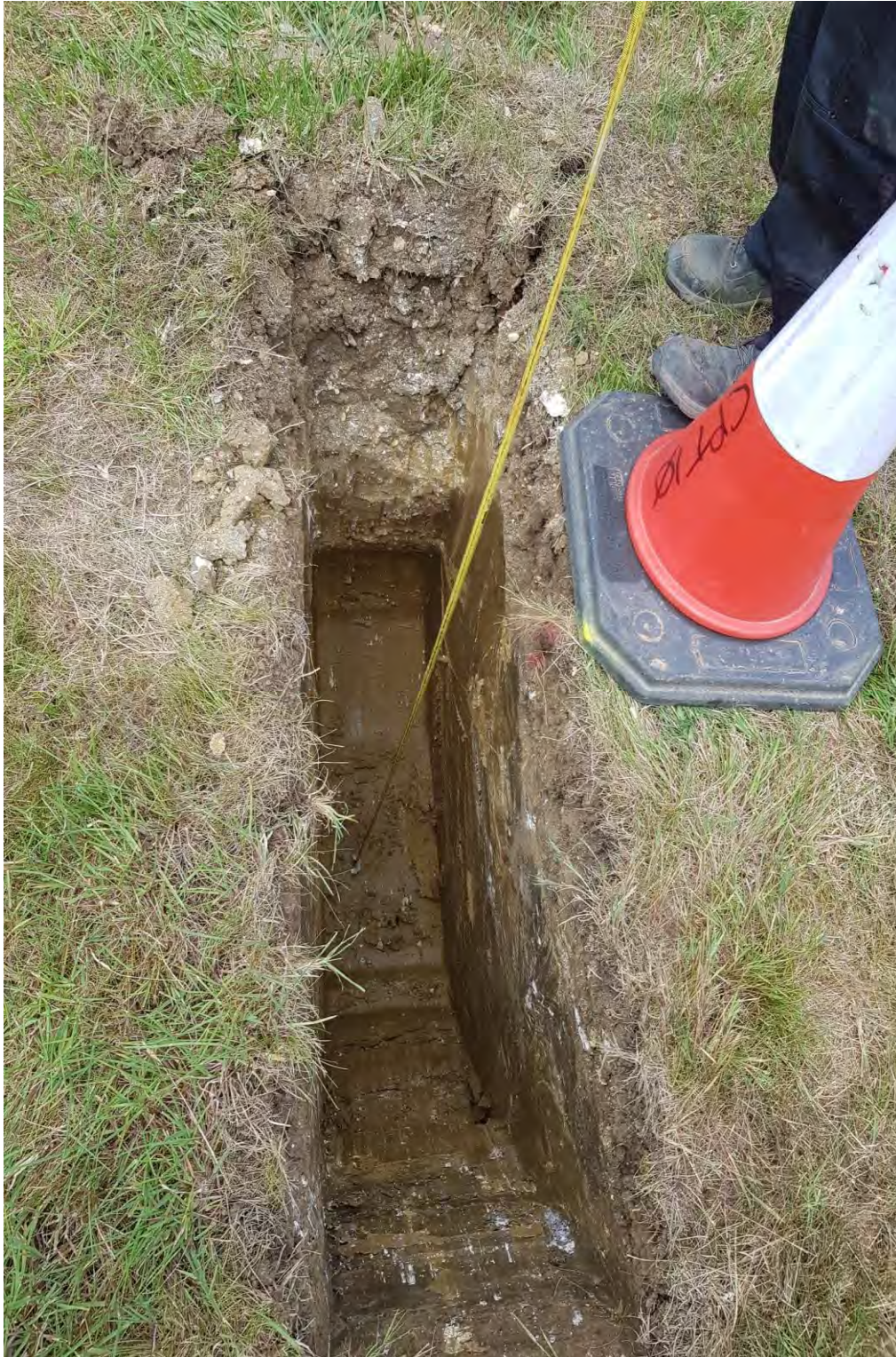
CPT10 GL to 1.50m Inspection Pit
