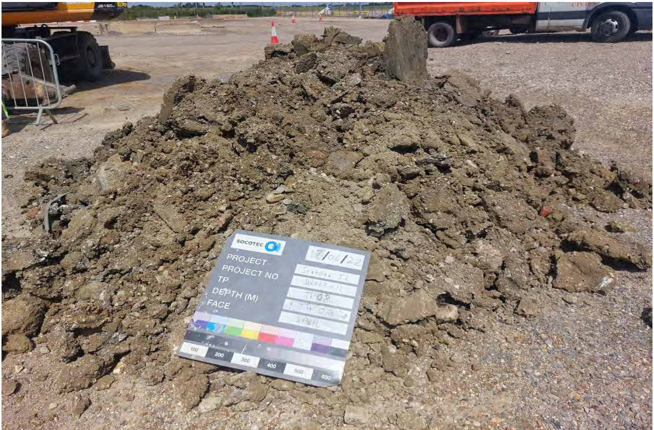
TP08 GL to 4.00m Spoil
