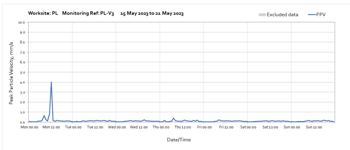
Note: High vibration levels measured at 12:00 on 15<sup>th</sup> May was due to compacting road surface works using roller in the vicinity of the monitor.
