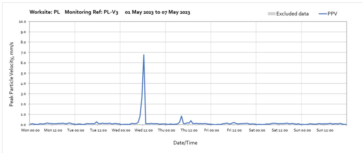
Note: High vibration levels measured between 11:00 and 12:00 on Wednesday 3<sup>rd</sup> May was due to compacting road surface works using roller in the vicinity of the monitor. The nearest receptor is further away and expected to be exposed to lower vibration levels.
