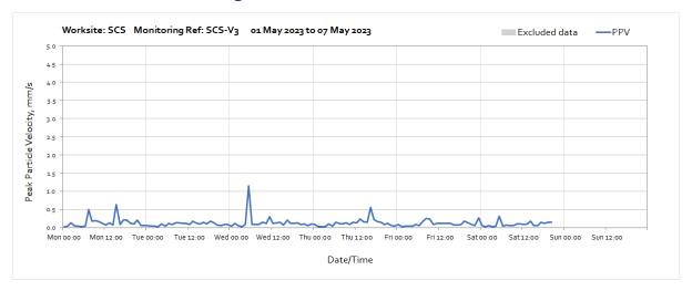
Note: Missing data between  $06^{th}$  May 21:00 and  $31^{st}$  May 23:00 due to failure of mains which powers the system so it stopped measuring.
