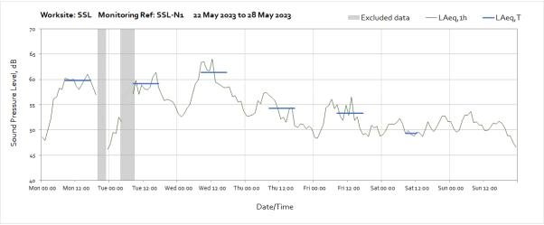
Note: Missing data between 22nd May and 23rd May 20:00 TO 08:00 due to malfunction of Micro SD which has been replaced.
