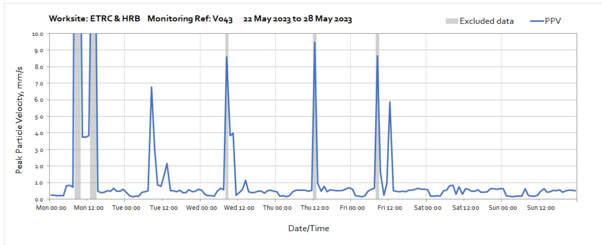
Note: High levels of vibration caused by works close to the monitor. Lower vibration levels anticipated at nearest receptor.
